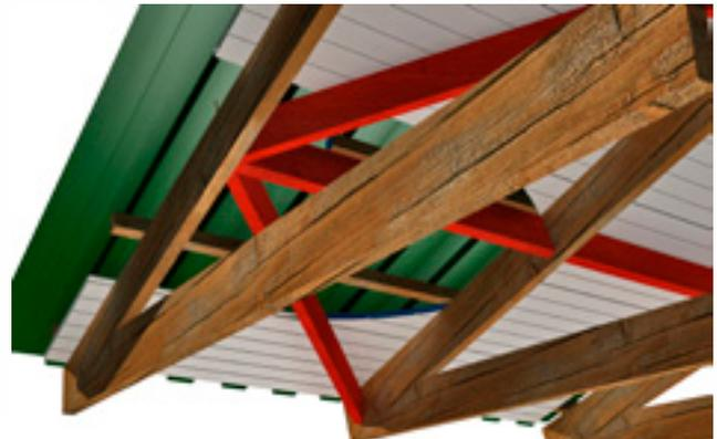
IsoBoard Over truss installation viewed from beneath, including additional top-chord bracing as required by truss designer.
