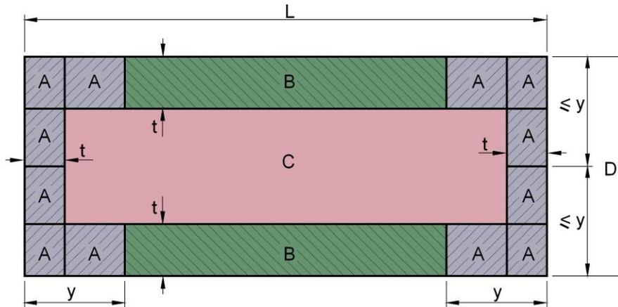
Note: A, B and C = zones on the roof subject to different wind pressures
