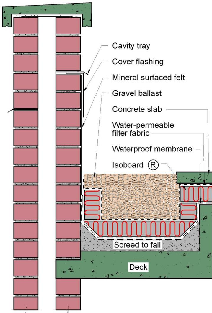
Figure 4: Parapet roof deck gutter detail – mastic asphalt
