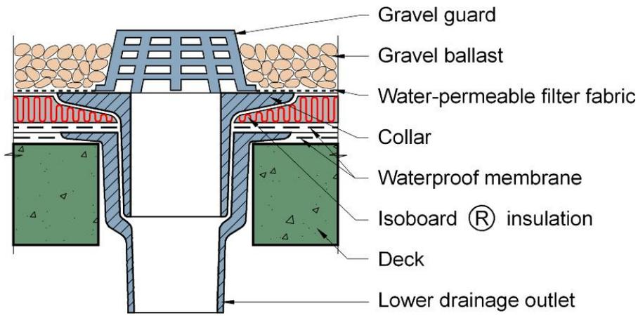
Figure 1: Gulley detail – two level drainage
