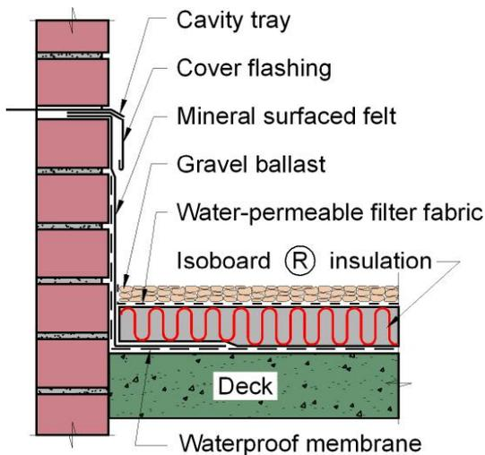
Figure 3: Parapet roof deck detail – bituminous waterproofing membrane
