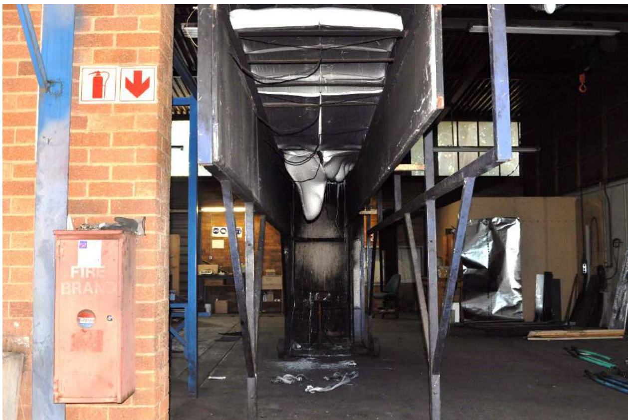
Figure 3.9: Test sample at conclusion of the SANS 10177 - 10 test
