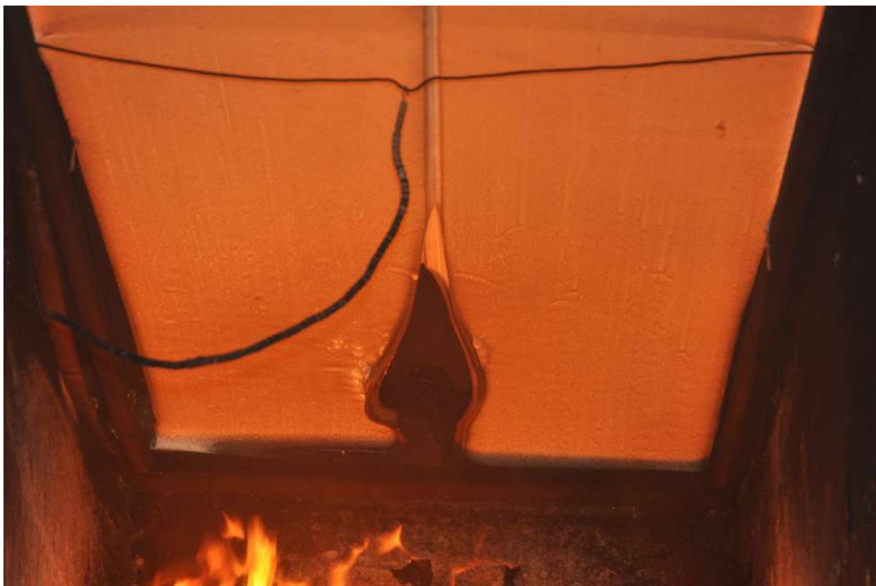
Figure 3.3: Discolouration and melting
