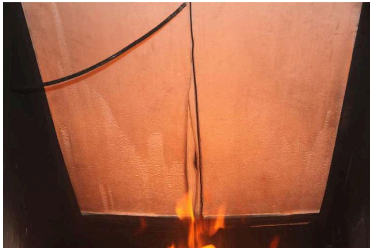
Figure 4.2.4.2: Shrinking of material visible and joint separating above Fire Source
