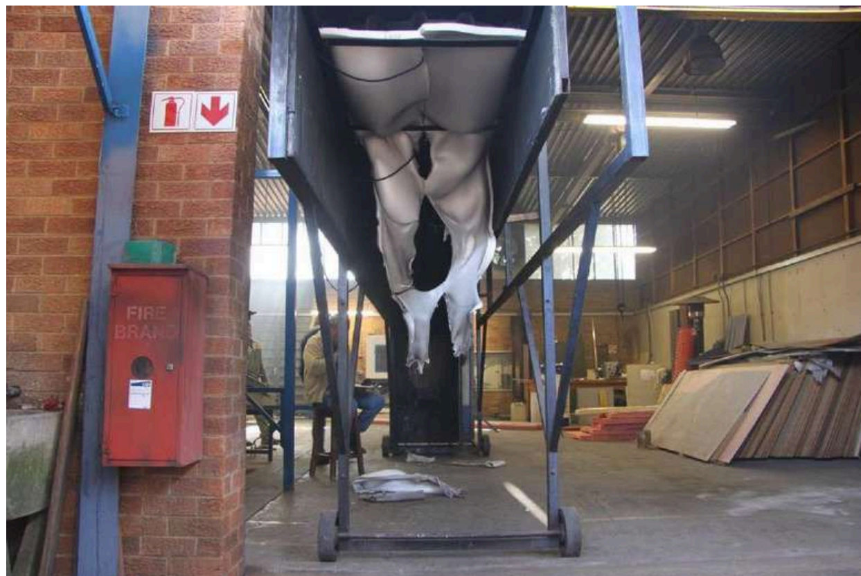
Figure 4.2.1.8: Test specimen at conclusion of SANS 10177 - 10 test
