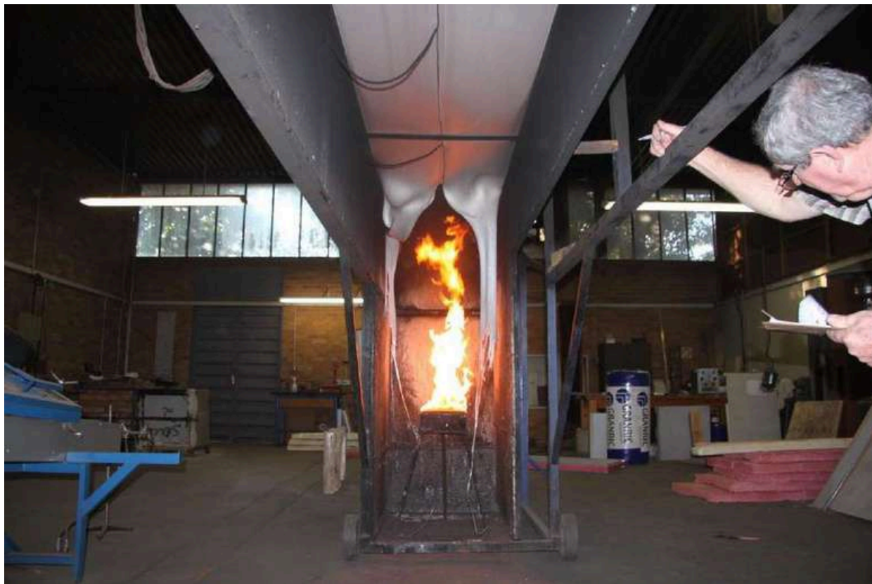
Figure 4.2.3.4: Material softening and flowing down in Ignition Source Area
