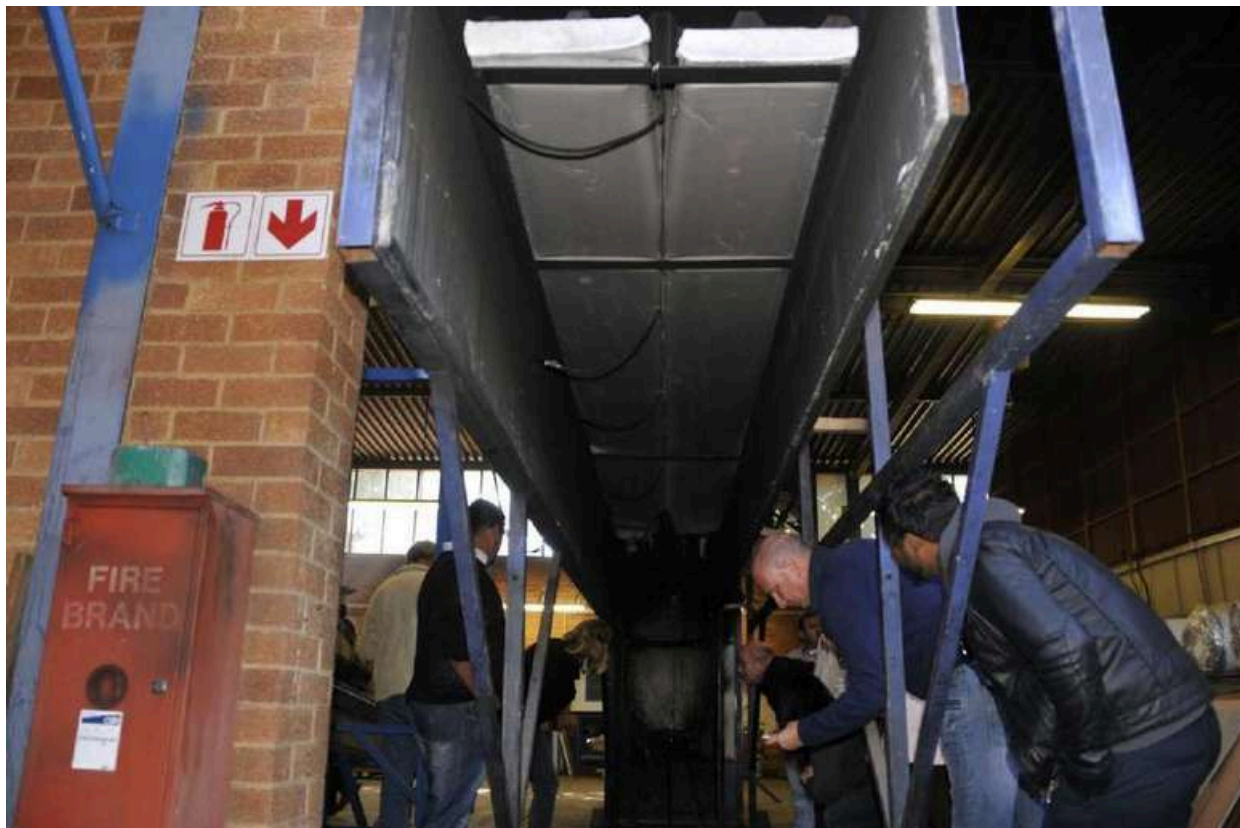
Figure 4.2.5.8: Test specimen at conclusion of SANS 10177 – 10 test
