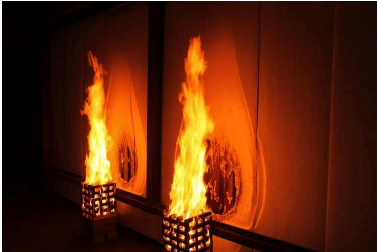
Figure 4.4.5: Molten material starting to flow down
