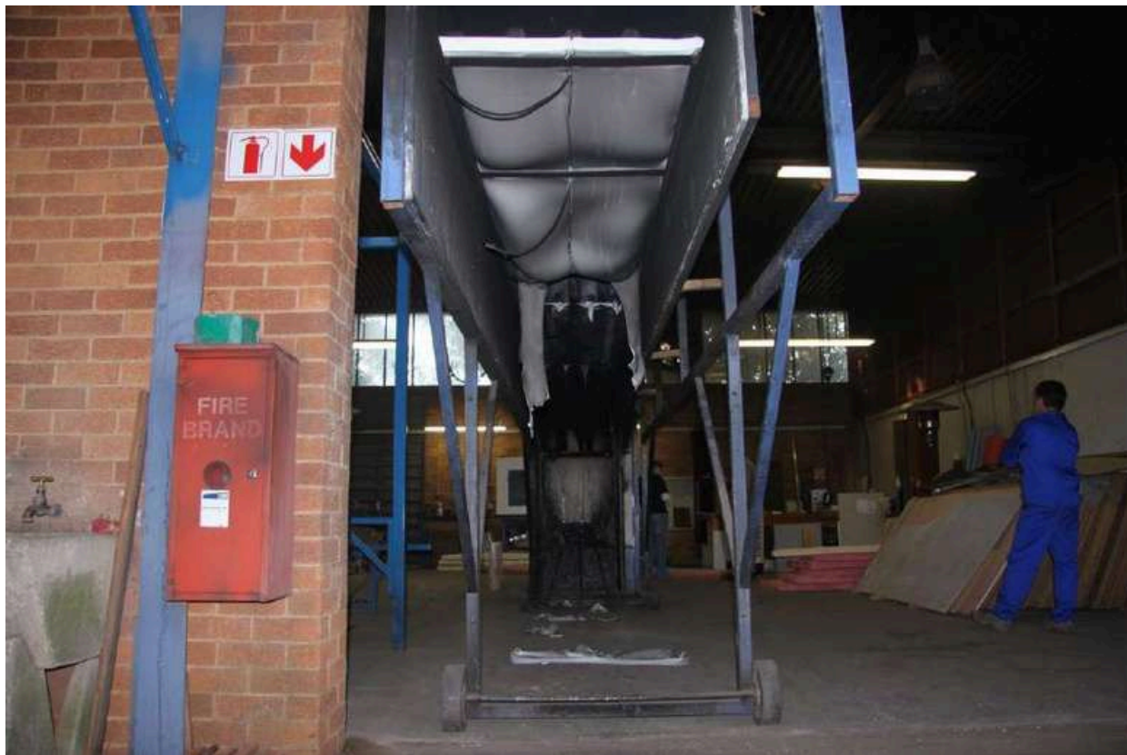
Figure 4.2.3.8: Test specimen at conclusion of SANS 10177 - 10 test
