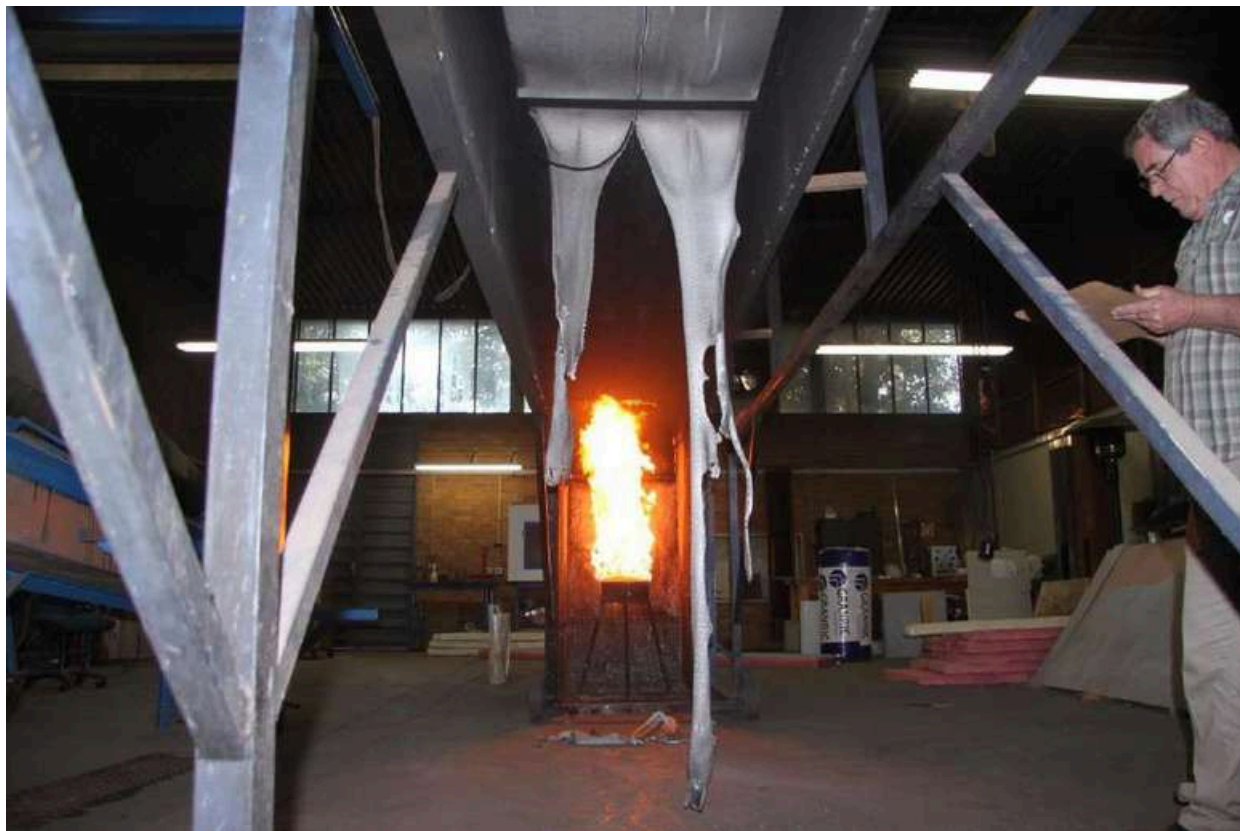
Figure 4.2.3.6: Material draping up to 4 meter mark
