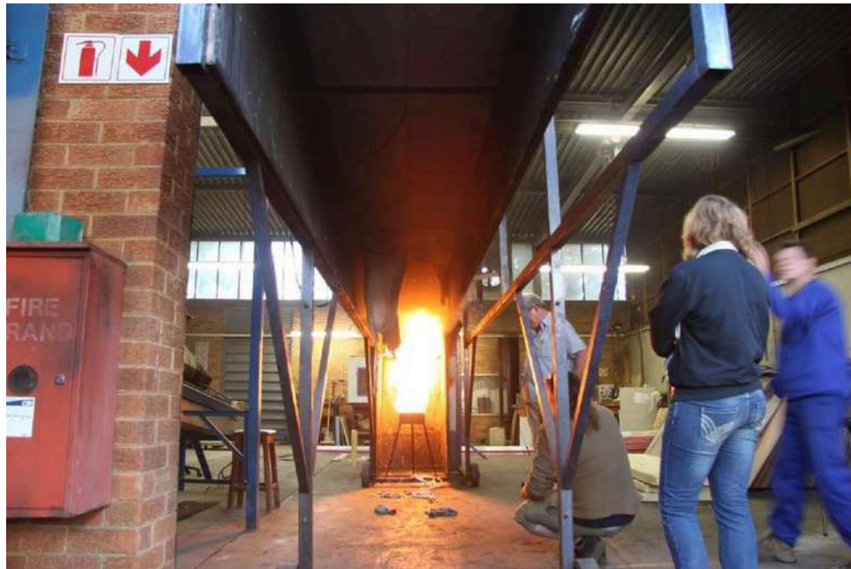
Figure 4.2.4.5: Material draping and dropping out up to 4 meter mark
