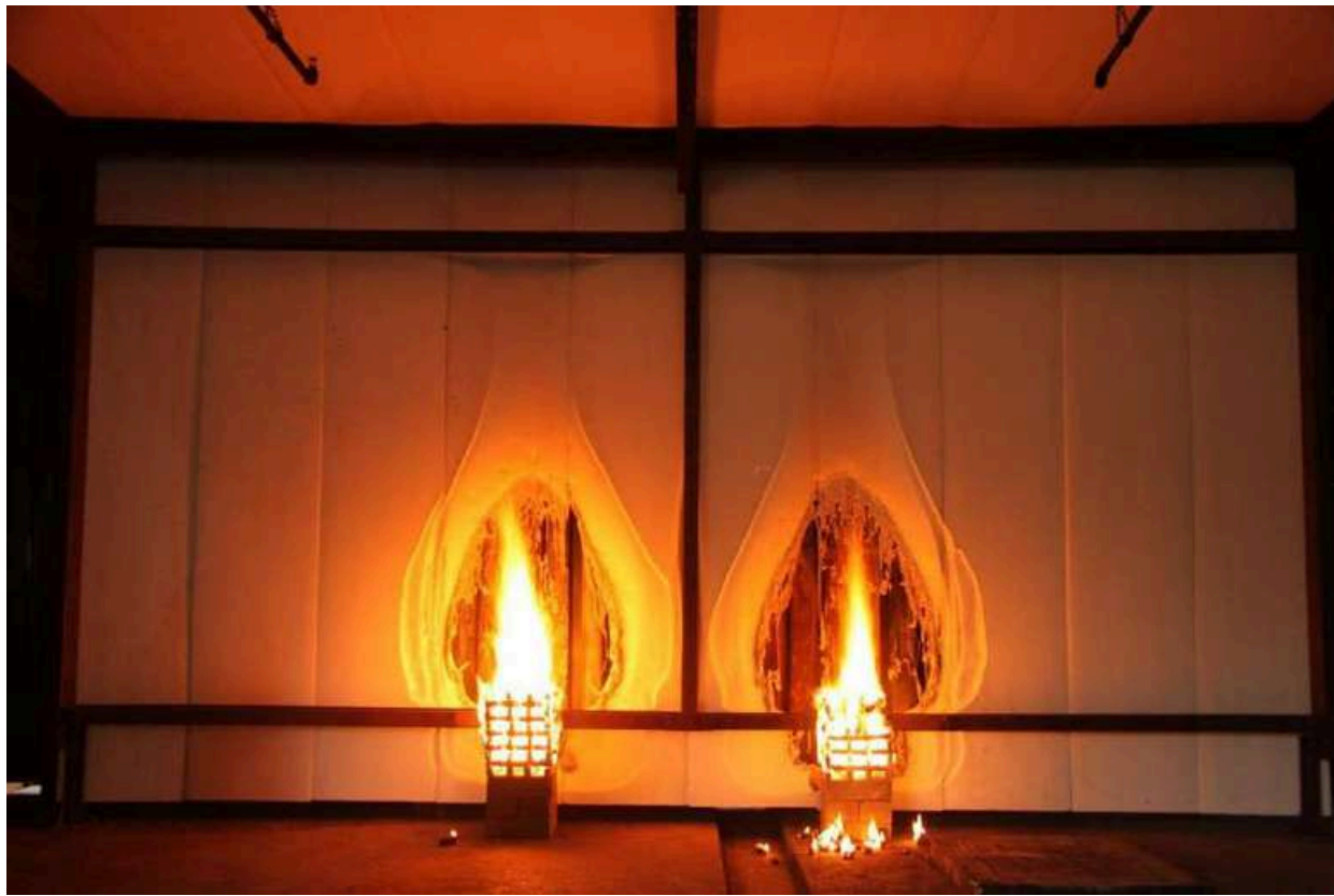
Figure 4.4.7: Cribs starting to collapse – No ignition occurred
