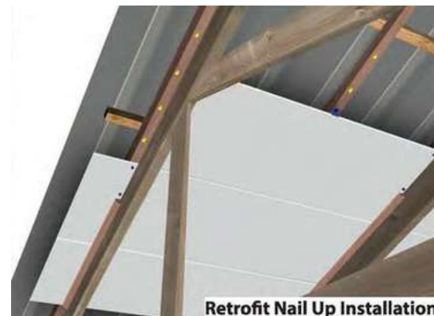
Retrofit nail up installtion
