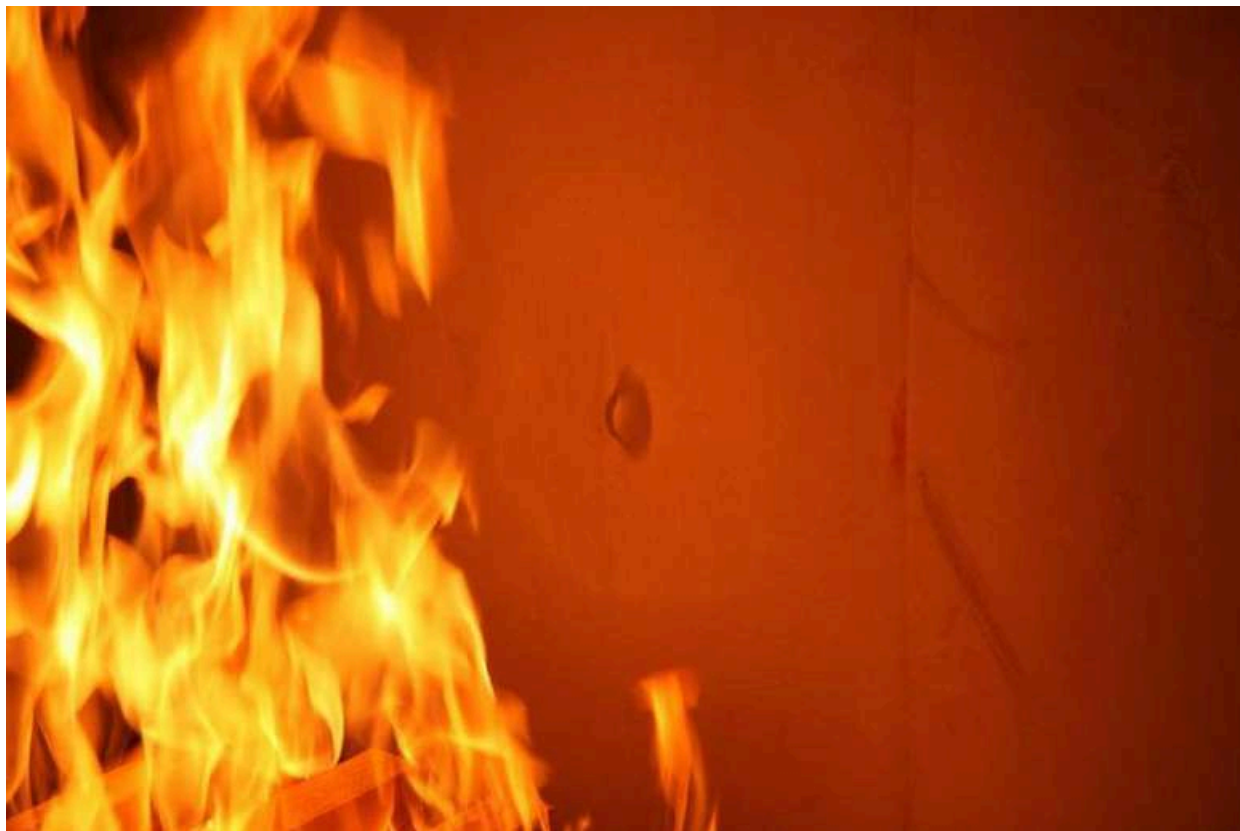
Figure 4.4.2: Material melting and bubble forming behind Crib
