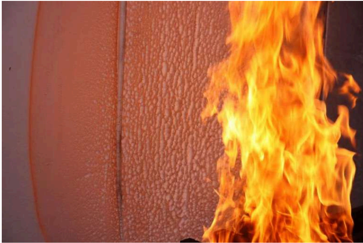
Figure 4.4.3: Coagulation of material behind Cribs
