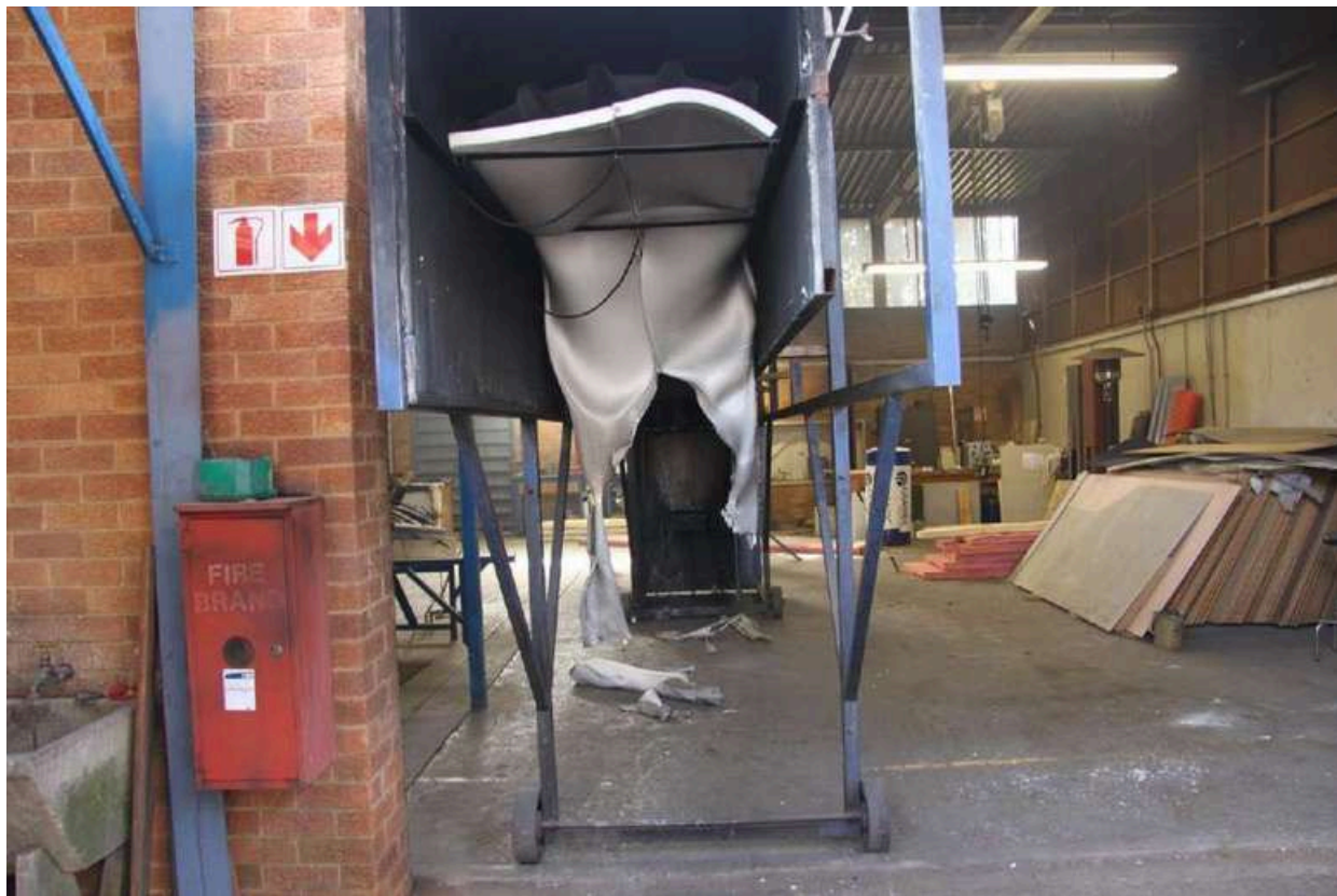
Figure 4.2.1.6: Test specimen at conclusion of SANS 10177 - 10 test
