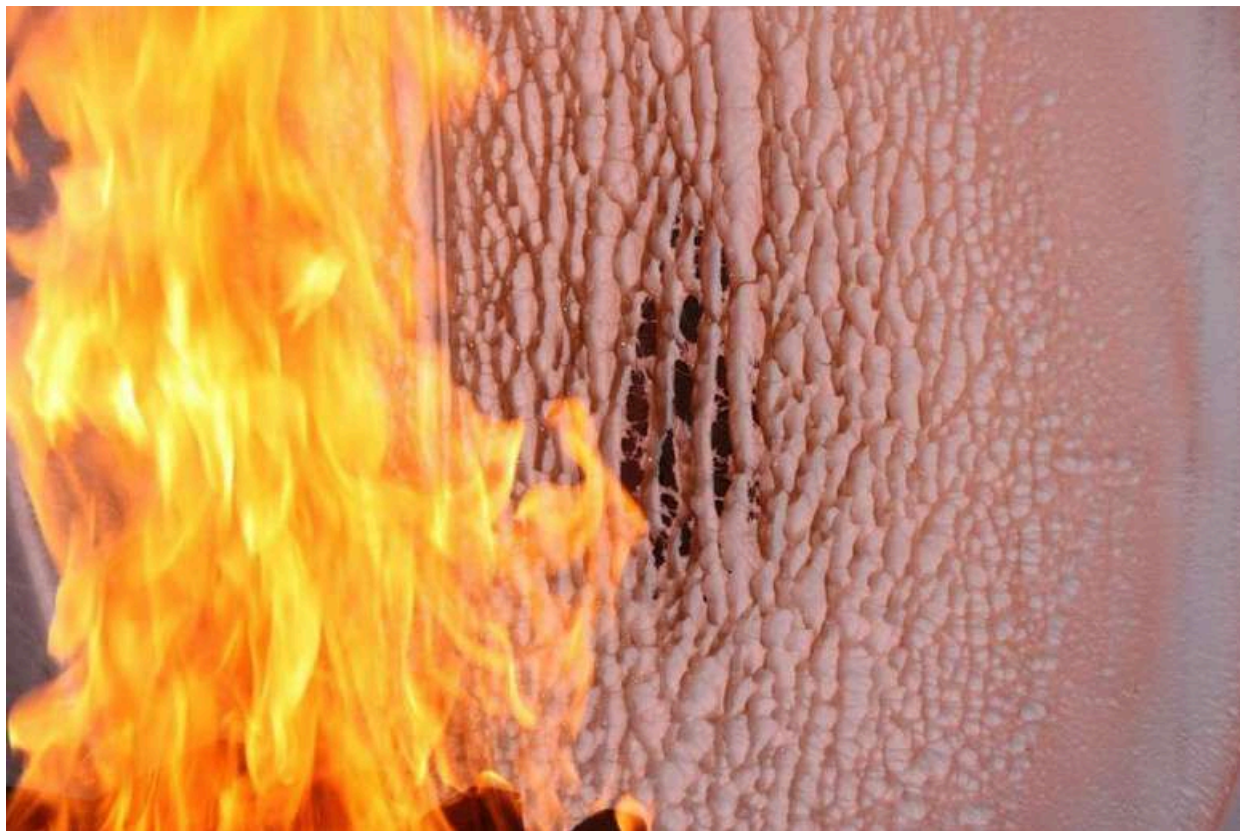
Figure 4.4.4: Coagulation of material exposing sheeting
