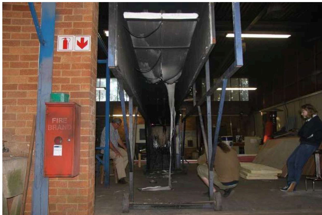
Figure 4.2.4.8: Test specimen at conclusion of SANS 10177 - 10 test
