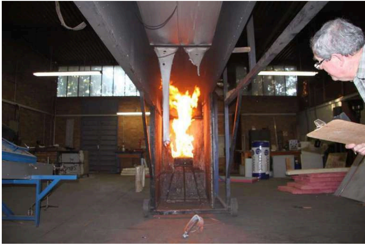
Figure 4.2.3.5: Material draping and dropping out up to 2 meter mark
