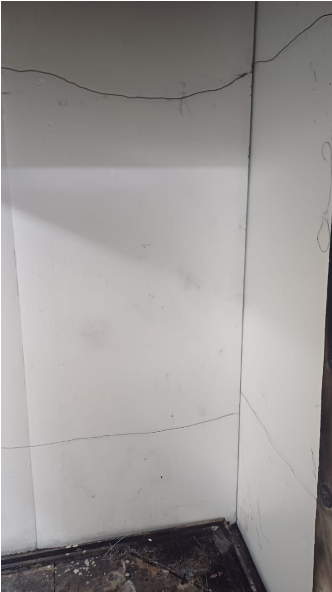
Image 1: Sample installed for a Single Burning Item test.
