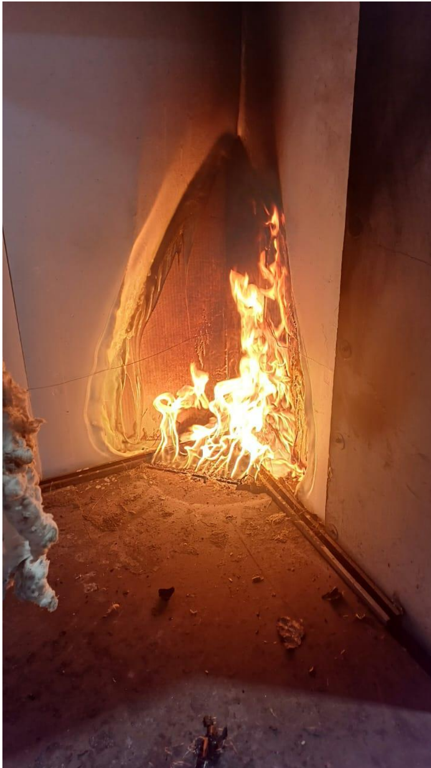
Image 2: Near the end of a Single Burning Item Test. No major flame spread or droplet development observed, with material mainly melting away from point of flame contact.
